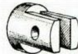
Fig. 2.—Fitting for taking the small end of connecting rod.
